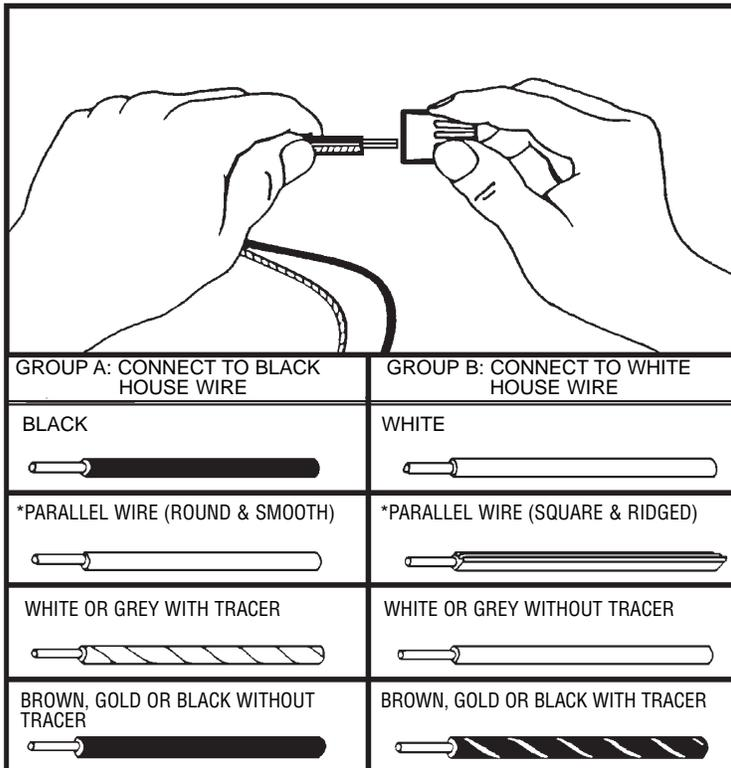
\*NOTE: When parallel wire is used, the tracer wire is square shaped or ridged, and the less tracer wire is round in shape or smooth. (See best when viewed from wire end.) To separate wires, grasp the ends of each wire and pull apart.
